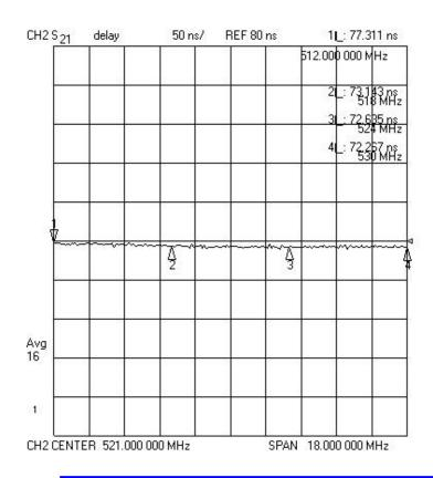
This plot is for a three channel wide UHF slot antenna, using our SFN™ slot technology. Even with the wide bandwidth of the antenna, our low Q coupling system functions in a very linear manner across all three channels. The differential group delay across any one channel is under 3 nS.
