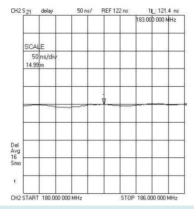
The plot above is for a top mounted high-band VHF elliptically polarized antenna. Even with the large pylon diameter, differential group delay is no more than 8.5 nS over the channel.
