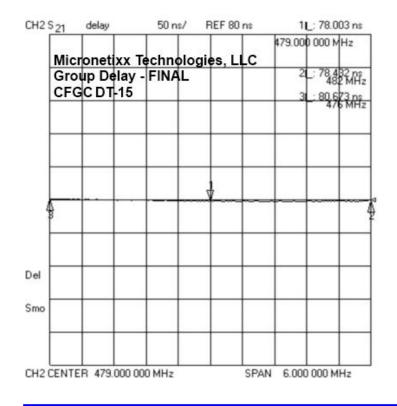
S<sub>21</sub> or Group Delay of a 6 bay UHF slot antenna. This antenna is elliptically polarized, and has a peak differential delay of only 2.5 nS across the channel. Our E/P antennas are fed in true quadrature phase, with all elements being DC grounded for optimal protection from lightning.
